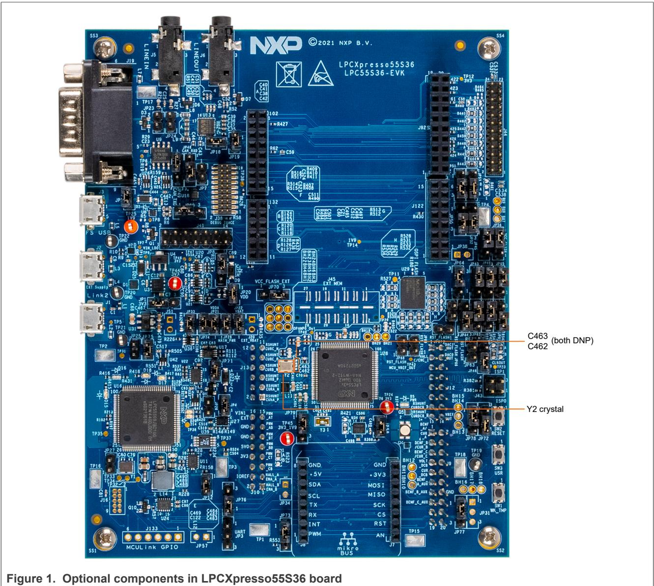
Figure 1. Optional components in LPCXpresso55S36 board
